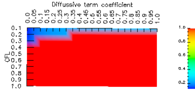
p=1 : Errors to discontinuous and Runge-Kutta(2) scheme
